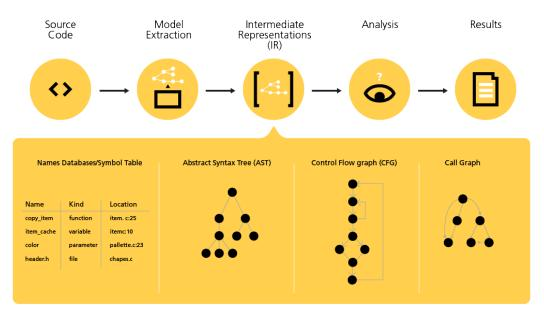
Figure 1. The architecture of an advanced static-analysis tool.
