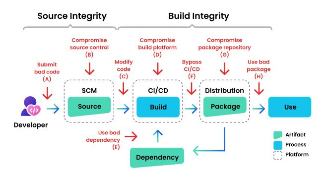
Any one of the links making up the software supply chain can be compromised. Indeed, there are as many possible supply chain targets as there are types of software. But current research highlights three main targets: dependencies, pipelines, and the combination of the two: pipeline dependencies.
